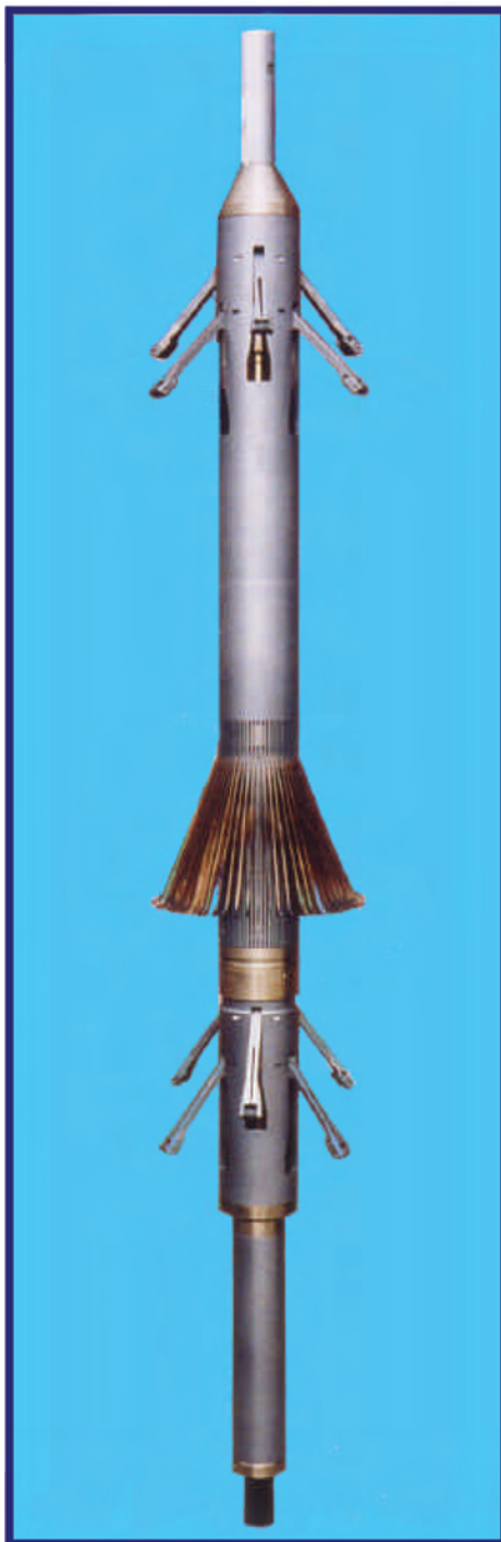
Fig. 3G.7—Multifingered caliper tool for deployment as a memory tool on slickline or as a surface-readout tool on monoconductor cable. This tool has 60 fingers, a 4-in. [100-mm] diameter, and a measurement range of 4.4 to 9.625 in. [114 to 245 mm]. It has a radial resolution of 0.005 in. [0.13 mm], a radial accuracy of \pm 0.03 in. [0.75 mm], and a vertical resolution of 0.23 in. [5.84 mm] at a logging speed of 3,000 ft/hr [914 m/hr]. Pressure and temperature ratings are 15,000 psi [103 MPa] and 350°F [177°C], respectively. Note the tool centralizers. (Courtesy of Sondex.)
